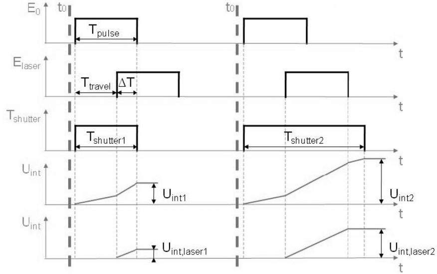
**Fig. 1.** Measurement Principle of the TriDiCam Technology
